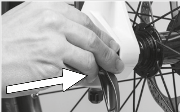
Figure 36: Pushing the quick release in
