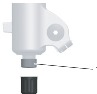
Figure 58: FOX rebound adjuster (1) on the fork
