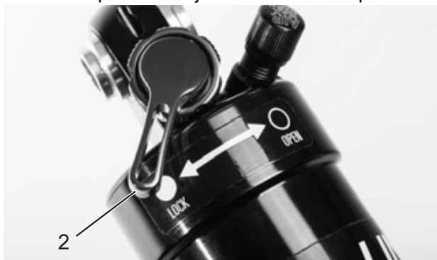
Figure 76: Suntour compression adjuster closed (2)
