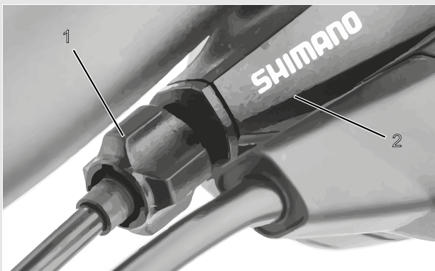
Figure 85: Adjusting sleeve (1) for the single-cable, cable-operated gear shift with shifter housing (2), example
