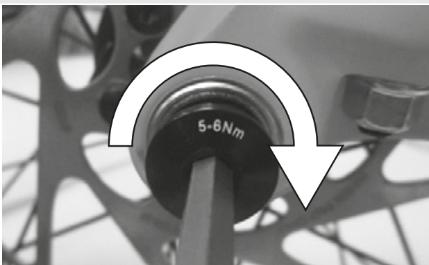
Figure 26: Tightening the securing screw
