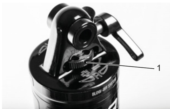
Figure 59: Suntour rebound adjuster wheel (1) on the rear frame damper
