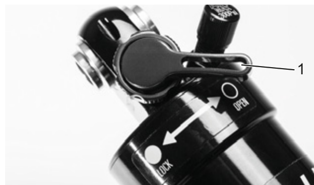
Figure 75: Suntour compression adjuster open (1)
