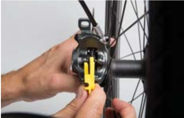
Figure 154: Checking the brake lining when fitted with the help of the transport safety wear gauge
