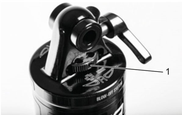
Figure 238: Suntour rebound adjuster wheel (1) on the rear frame damper
