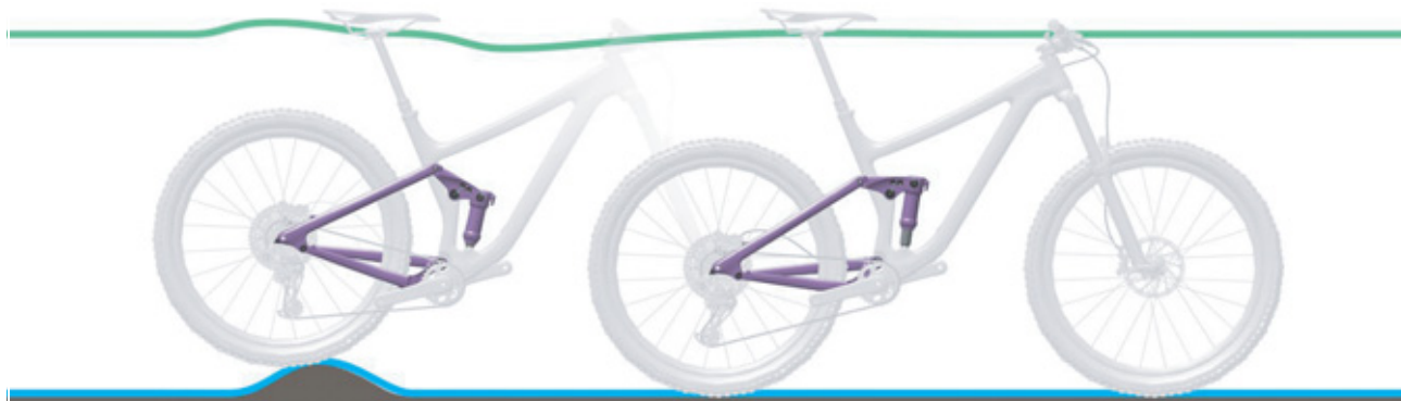
Figure 117: Optimum rear frame damper ride performance over bumps
