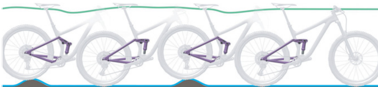
Figure 115: Optimum rear frame damper riding performance
