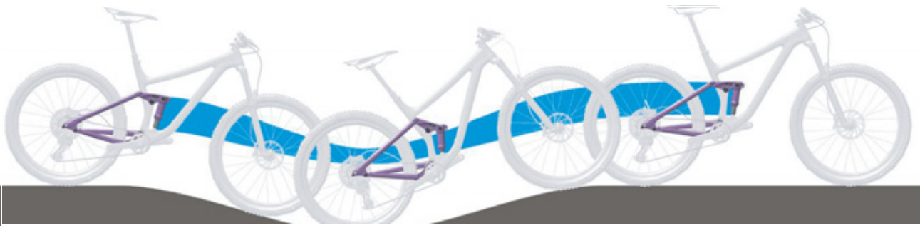
Figure 239: Excessively soft suspension in the rear frame damper on hilly terrain
