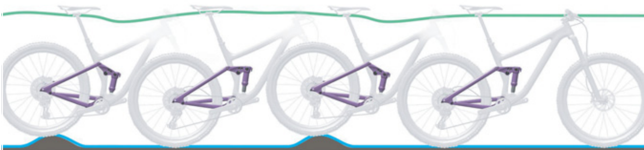
Figure 15: Optimum rear frame damper ride performance
