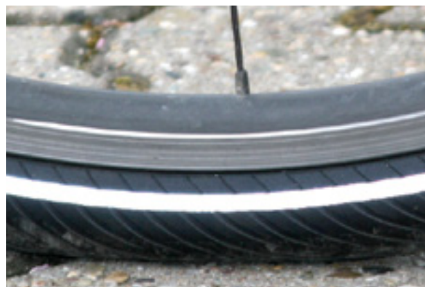
Figure 102: Correct tyre pressure. The tyre is barely deformed under the load of the body weight
