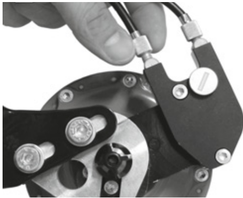
Figure 158: The tension adjuster on Rohloff hub versions with external switch control is located on the cable box positioned on the left-hand side
