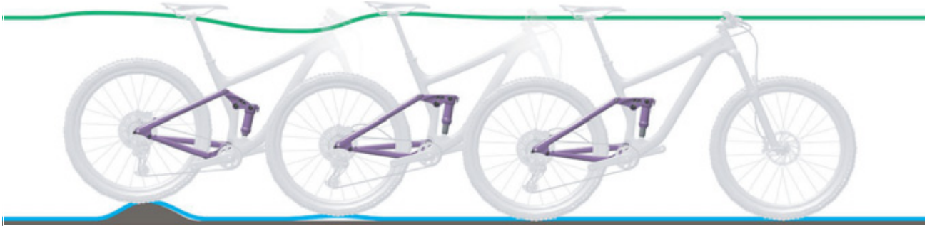
Figure 235: Rear frame damper rebounding too quickly
