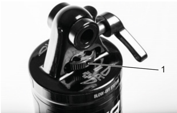
Figure 236: Suntour rebound adjuster wheel (1) on the rear frame damper
