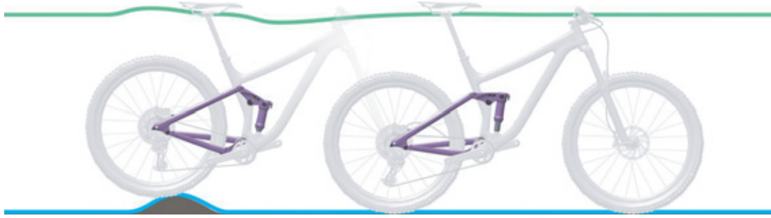
Figure 17: Optimum rear frame damper ride performance over bumps
